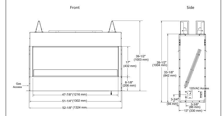
When utilizing the optional drain pan(ODLANAIG-48DP), please refer to installation manual for details.
